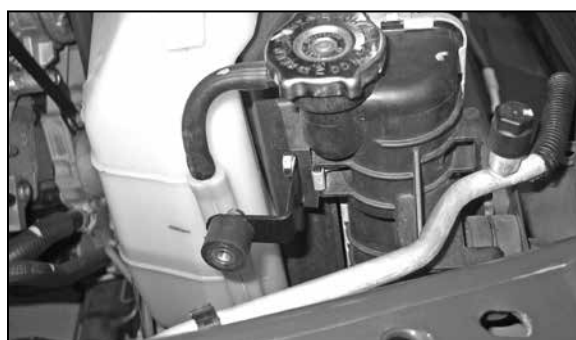
16. On 2008 & earlier vehicles install the "L" bracket (26607) onto the fan shroud with the provided 8mm bolt and washers.
