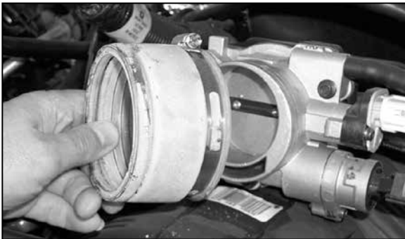
8. On 2002-2007 model year vehicles, loosen hose clamp that retains the rubber hose to the throttle body then remove as shown.
