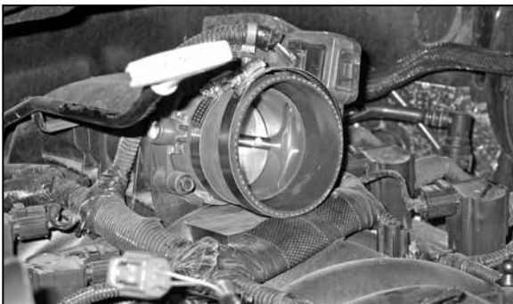
8a. Install the provided silicone hose (08051) onto the throttle body and secure with the provided hose clamp.
