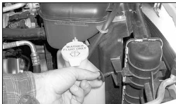
15. On 2008 & earlier vehicles, remove the 13mm bolt from the upper fan shroud as shown.
